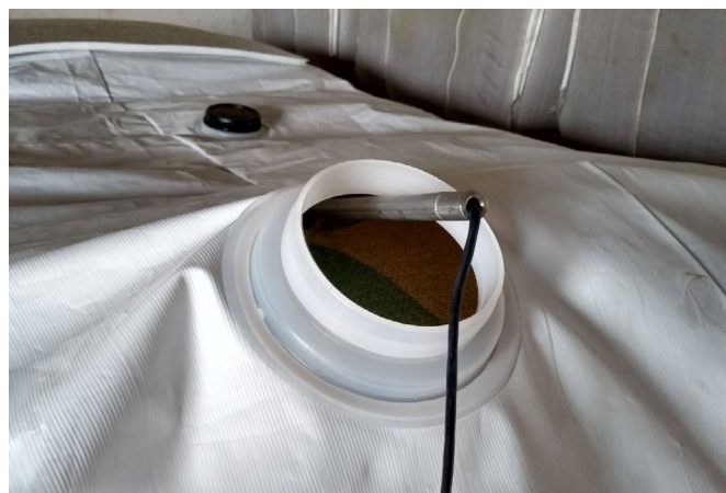
Figure 2: Probe positioned through an air outlet of the cocoon, measuring the grain mass at approximately 0.5 m below the top of the pile.
