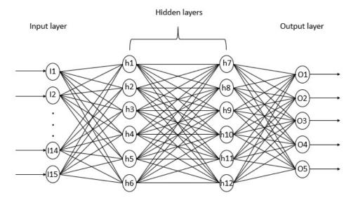
Figure 3: Architecture of the neural network model.
