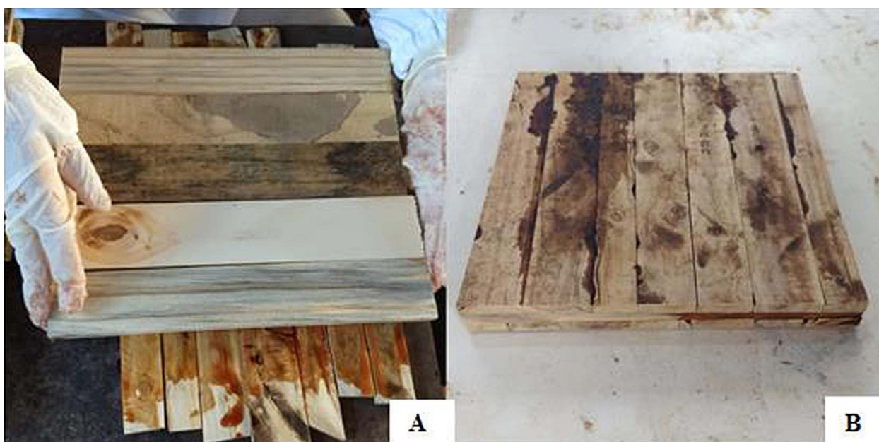
Figure 1: Manufacture of the CLT panel: (A) bonding the veneer and (B) finished panel.
