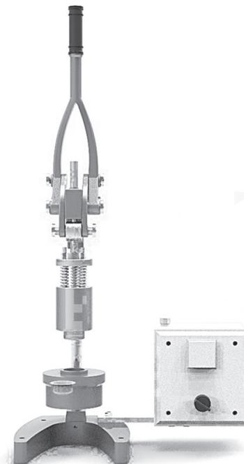
**FIGURE 1**- Laboratory prototype of coffee pod packaging with a single chamber.
